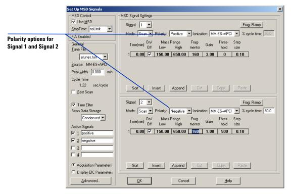
Figure 21 Positive/Negative polarity switching using Set Up MSD Signals dialog box
